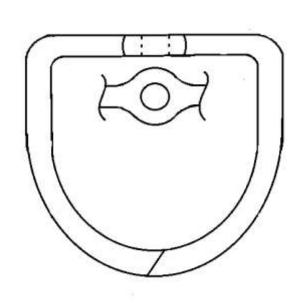
5. Bend toes of prepared material around, successfully weld the two ends together. Blend area back into apparent section (8mm round) **ANY** wastage to be taken into consideration when judging.
