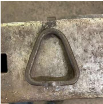
6. FINISHED ARTICLE; Once fully welded. Form the sides of the shackle, this will replicate the desired shape of the sample.
