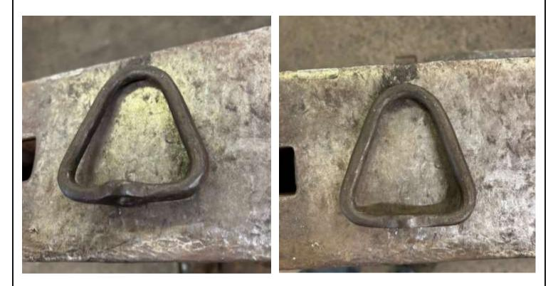
6. FINISHED ARTICLE; Once fully welded. Form the sides of the shackle, this will replicate the desired shape of the sample.
