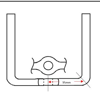
4. Bend the required bends. Centre of the bend desired should be **35mm** from the centre of the punched hole. Prepare ends of bar for fire welding.
